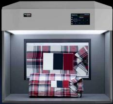
VisionView offers immediate improvement in cost and efficiency by including the latest generation Ezio monitor in the new VeriVide all-LED tunable UltraView light booth. It is a versatile tool that enables users to combine the advantages of both visual and digital assessment.
