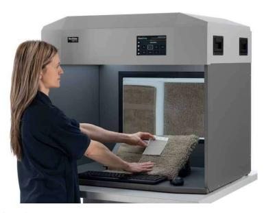
In the same operation, physical samples can be assessed visually in precisely controlled LED viewing conditions and compared with a digital standard image taken in a DigiEye imaging system.
