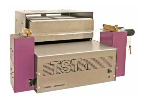
Changes in length and shrinkage force at specified temperatures are two dominant quality parameters for films, nonwovens, laminated products and fabrics.
