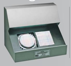
The Pilling Assessment Viewer (PAV) for the textile market has been developed with the help of a major textile company in accordance to BN EN ISO 12945 standards incorporating all 3 parts and adopting the following test methods...
