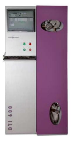
Filament characteristics such as molecular orientation, dyeability, shrinkage and shrinkage recovery are important quality parameters, but usually their determination is time consuming and expensive. These characteristics are straight connected to the draw tension or draw elongation, which are directly related to shrinkage force and shrinkage - but measured on a running yarn. That means faster measurement, information about variation and better useability of the results.
