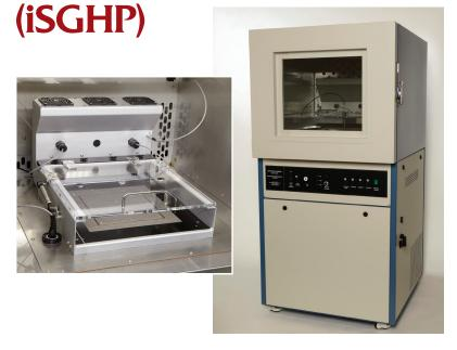
The Sweating Guarded Hotplate, or "Skin Model", is used to produce accurate, repeatable measurements of thermal resistance (Rct) and vapor permeability (Ret) for textiles as per ASTM F1868, ISO 11092, and ASTM D1518.
