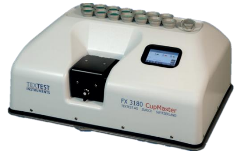
FX 3180 CupMaster Water Vapor Transmission Rate Tester
