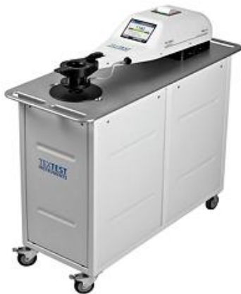
FX 3300 LabAir IV Air Permeability Tester
