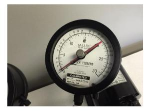
• Our gauges scale from 15 to 300 PSI and are precisely calibrated to 0.5% full scale.
