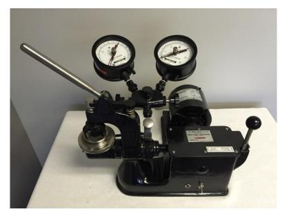
Since its invention in 1887, the Mullen<sup>®</sup> Burst Tester has been the industry benchmark for measuring the burst strength of paper, paperboard, nonwovens, textiles, plastics and medical materials. Mullen<sup>®</sup> is cited in many TAPPI, ASTM, INDA and International Standards – and when it comes to quality control, our tester is an integral part of any well-equipped lab.
